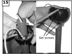
Thread wires through half ball, put ball back over downrod and replace pin then tighten the two set screws
